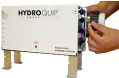
Align the other studded clamp and attach to the other slide bracket. Now determine the proper alignment for the heater and tighten the nuts and clamps
